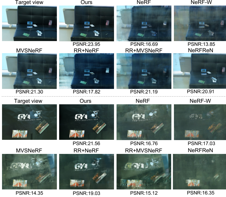
Figure 4: From left to right: the target view, our results, the results obtained by NeRF [1], NeRF-W [7], MVNeRF [10], RR+NeRF [1], RR+MVNeRF [10], and NeRFReN [32]. The target views in the two scenarios (scenes with detachable glass, captured with the similar setup as [6]) are obtained by removing the glass, and are compared with the results as ground truth for PSNR values shown below each image. Please zoom in for more details.
